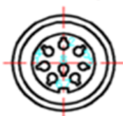
B: AISG Connector (Female)
